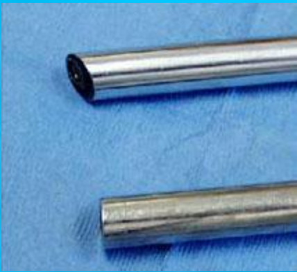
The HOPKINS rod lens system employs special glass rods
